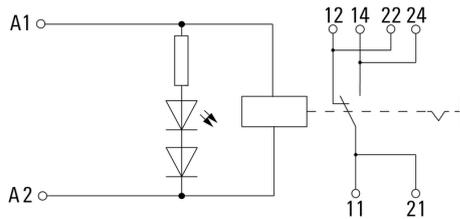
For full continuous current (16 A), the wire terminals 11 with 21, 12 with 22 and 14 with 24 must be bridged with a wire  $\geq 1,5 \text{ mm}^2$  at the socket.
