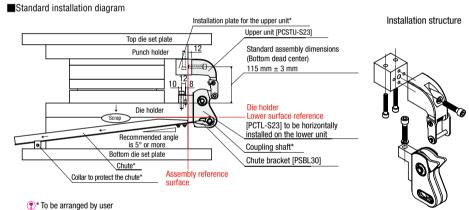
A rod can be used to support the chute; however, it is recommended that you use a rotating part such as collar to reduce of wear.
